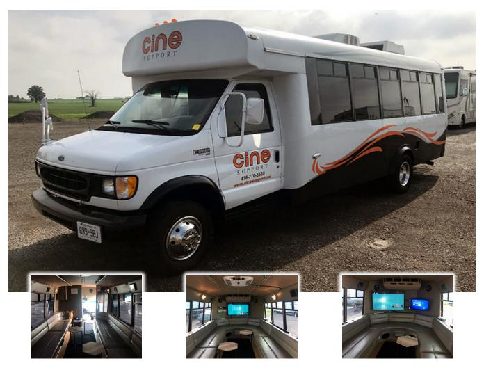
The "Client Bus" comfortably seats 10 people with two monitors situated at the rear of the bus for clear sight lines. The bus is equipped with a Honda 3000IS generator allowing to work autonomously from the main unit. The bus is also equipped with tails to tie into the main set generator. There are numerous power stations located throughout with small work tables for laptops. The newly installed AC/HEATING unit provides comfort for all seasons.
